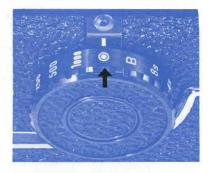
Since the PD Prism Finder utilizes the battery in the camera body, a timer is incorporated into the meter switch of the PD Prism Finder to prevent unnecessary electrical consumption.
