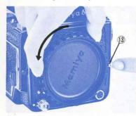
While depressing the lens release button (13), turn body cap counterclockwise until the red dots are aligned and lift out.
