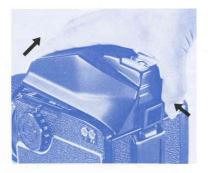
2. While pushing in on the release button with your thumb, lift the finder off the camera body.
