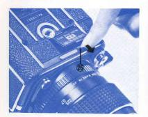
The Mamiya M645 uses one 6V silveroxide battery 4SR44 (Eveready No. 544, UCAR 544, Mallory PX28 or equivalent) or alkaline battery 4LR44.
