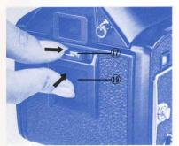
1. While gently pushing in on the memo clip (19), move the back cover latch (17) in the direction of the arrow and the camera back cover will open.
