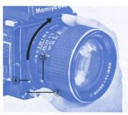
While aligning the two alignment dots (33 & 4), insert lens into camera body. Then twist lens clockwise until it clicks and locks into place.
