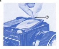
Remove the finder, grasp the focusing screen lug (2), pull up, and lift out. To replace screen, gently insert and lightly push it in on both sides until it stops.
