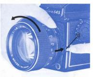
While depressing the lens release button (13), grasp the part of the lens barrel that has the depth-of-field scale (32) and alignment dot (33), and twist the lens counterclockwise until it stops. Then lift out.
