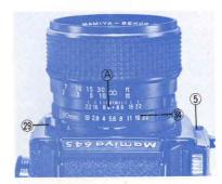
Set the desired f/stop on the aperture ring (34) by aligning the f/number with the red reference dot (A). (The aperture ring has a click stop for each f/stop. In-between clicks can also be used.)
