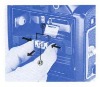
2. While squeezing in on both sides of the release latch (37), pull the roll-film insert out of the camera body. Place the film insert on a table making sure that the film type index (42) is not upside down. Then pull out and lower the spool clips found on the left-hand side.
