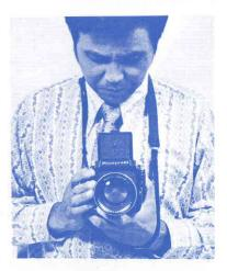
When hand-holding the camera with the waist-level finder attached, adjust the length of the neck strap to take up all slack and support the camera gainst the body. As accessories, Mamiya offers a selection of hand grips which not only help to eliminate camerashake, but are also convenient for carrying the camera.
