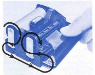
6. Gently pull out some of the leader paper, pulling it over and around the pressure plate. Then insert the tip of the leader paper into the slot of the take-up spool.
