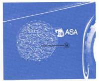
**4.** Pull out and turn the ASA dial (B) until the appropriate ASA number appears in the window.
